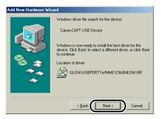
Installation of the USB class driver starts.
